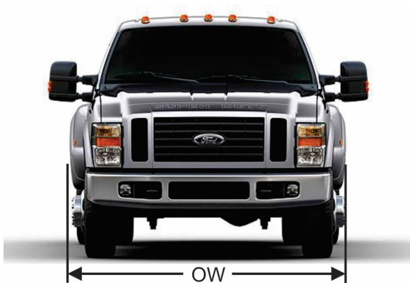
Figure 9 - Overall Width Includes Add-on Fender or Wheel Flares
