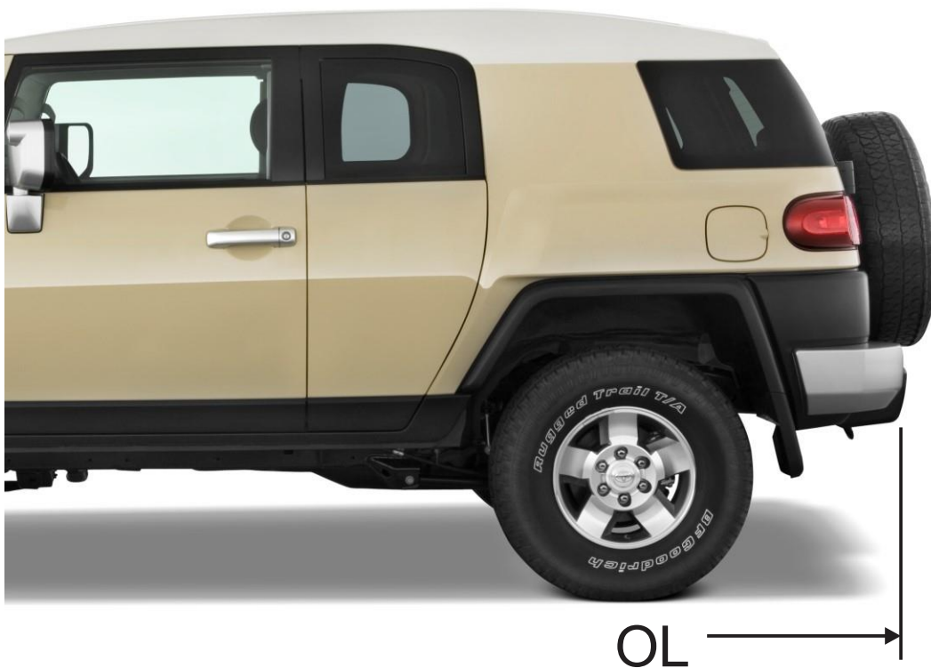
Figure 7 - Overall Length Excludes Rear Mounted Spare Tire
