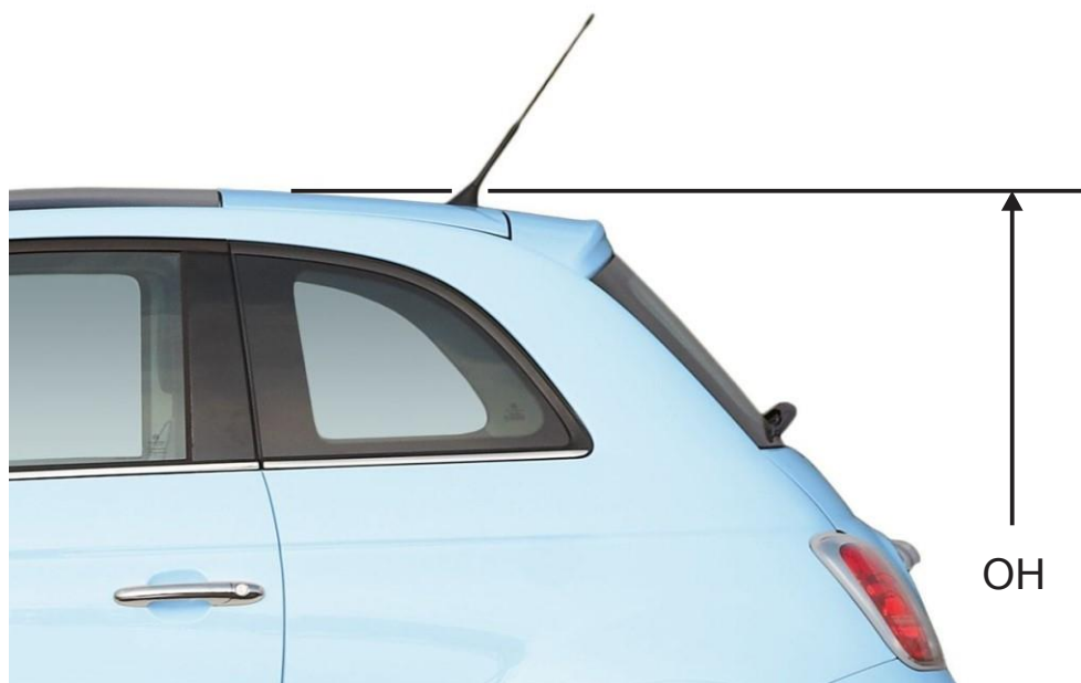
Figure 11 - Overall Height Excludes Antennas and Optional Equipment
