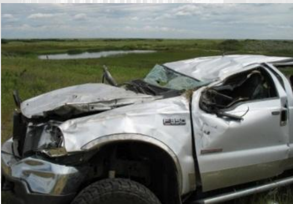
Structural damage to a pickup truck's roof following a rollover
