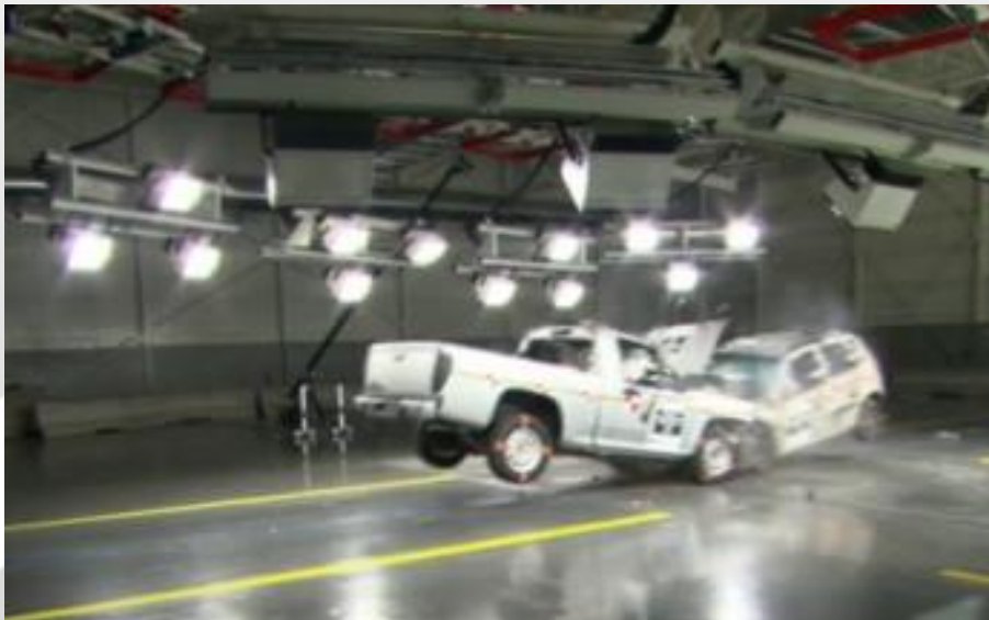
An actual crash test shown in the film, involved a pickup truck travelling at 71 km/h and impacting a hatchback travelling at 56 km/h.
