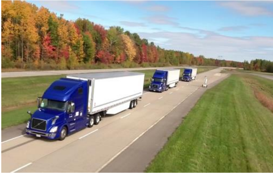
Fuel economy testing of a three-vehicle, truck-platooning system.
