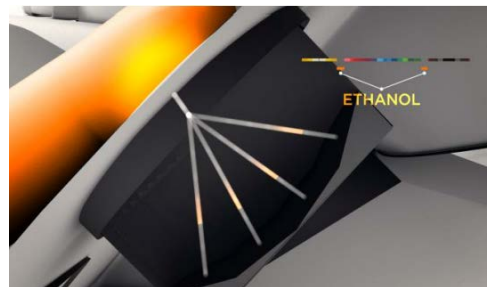
Takata-TruTouch non-invasive alcohol sensing system using near-infrared spectroscopy on the driver's finger
