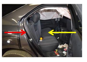
Seatbelt loading / front seatback contact + Cargo loading (rear seatback)
