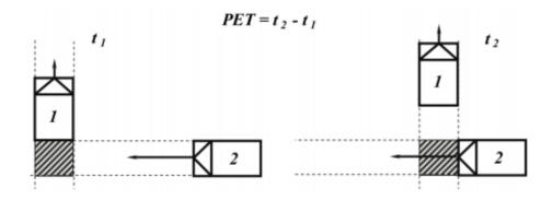
**Gap time:** how much time elapses after Vehicle 1 leaves the encroachment zone before Vehicle 2 enters the zone?
