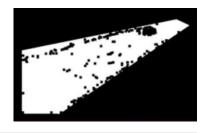
Step 3 Object grouping: A heuristic algorithm brings together features based on speed, proximity, and share geometric edges. Objects may then be classified as vehicles, pedestrians, cyclists, etc.
