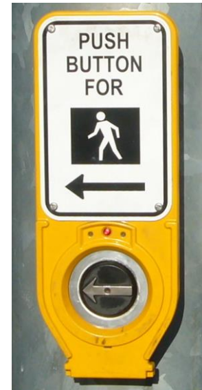
Accessible pedestrian signals
