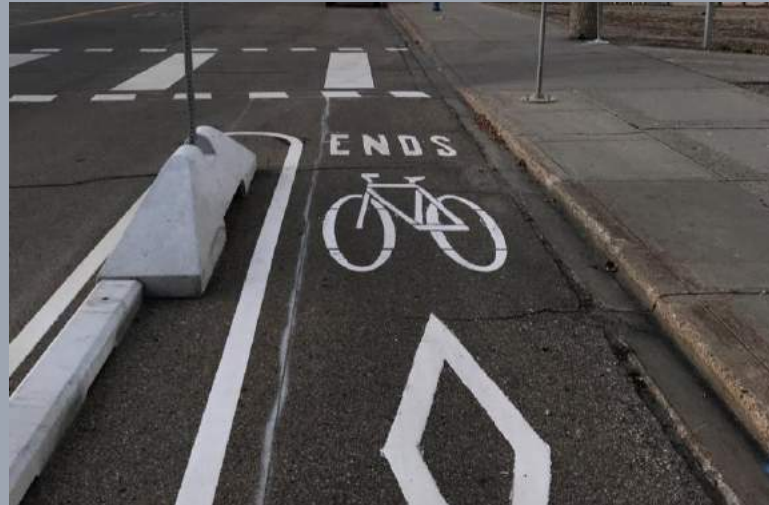
On-road uni-directional protected bicycle lane
